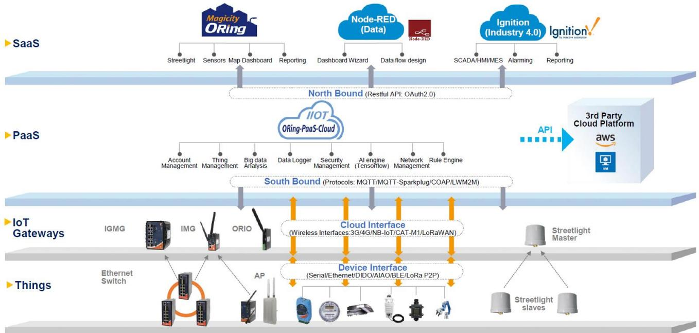
Above architecture picture shows typical application and use case scenario for ORing IoT system. IoT Gateways are responsible for providing transparent connectivity between end-devices and South Bound interface of the Cloud platform. Once the data reaches the Platform it can be stored securely and analyzed. Applications on the top of the system provide HMI and Dashboards for data visualization, reporting, alarming, historian and device location.
